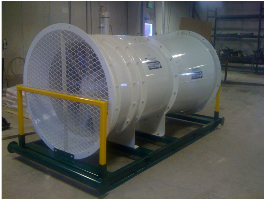
Figure 7.6. Completed skid with the mounted booster fan
