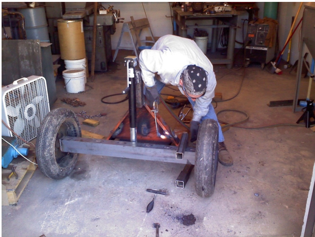
Figure 7.7. Removable lifting axle assembly
